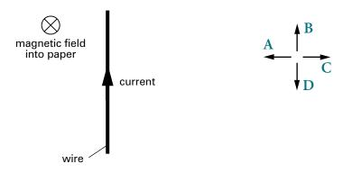
Which arrow shows the direction of the force on the wire?
