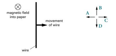
Which arrow shows the direction of the induced current in the wire?
